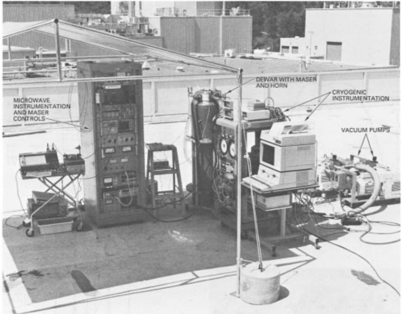
Fig. 7. Rooftop system test setup.
