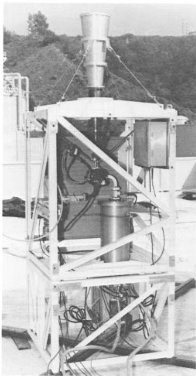
Fig. 6. The X-band test package in the 22-dBi horn configuration for testing at JPL.
