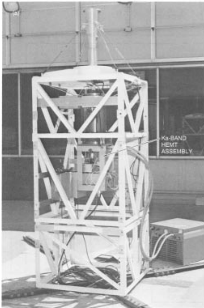
Fig. 2. Ka-band test package in its 29-dBI horn configuration for testing the system on the roof of the Telecommunications Building: (a) showing Ka-band HEMT and (b) showing Ka-band ambient-load thermal reference and downconverter.
