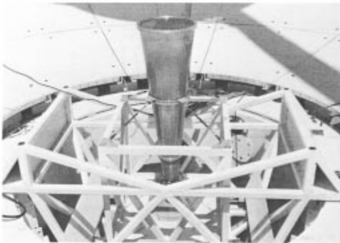
Fig. 3. The Ku-band test package mounted at F1 in the 29-dBi horn configuration.
