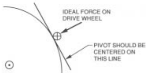
Fig. 4. Directions of force of the modified design for improved acquisition accuracy.
