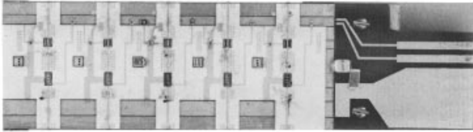
Fig. 8. Amplifier module containing the 100-mW 32-GHz amplifier and 50- \Omega through line.
