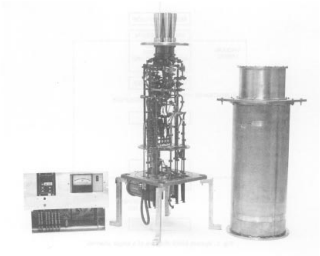
Fig. 2. The front end with vacuum vessel and instrumentation.
