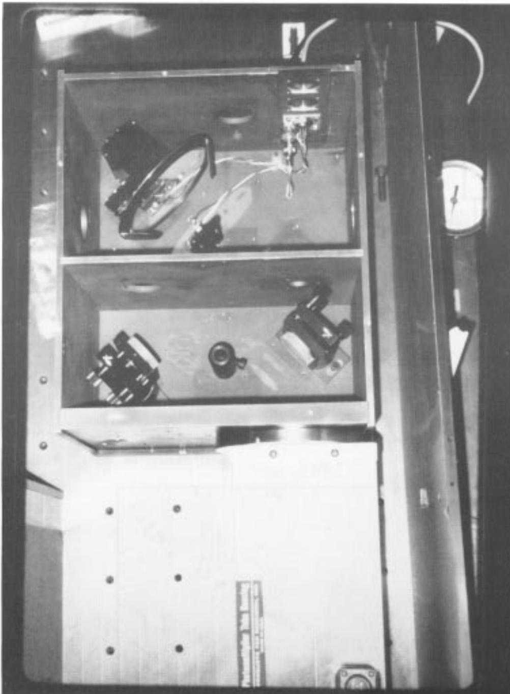
Fig. 1. Photograph of T/R switch with top cover removed. The 10-cm holey mirror consisting of a dielectrically coated surface is shown in the right chamber. The two relay mirrors that direct the return signal to the photomultiplier tube are shown in the left chamber tube. A polarizing beam splitter at SOR and a holey mirror at TMO were used to relay the return beam to the detector.
