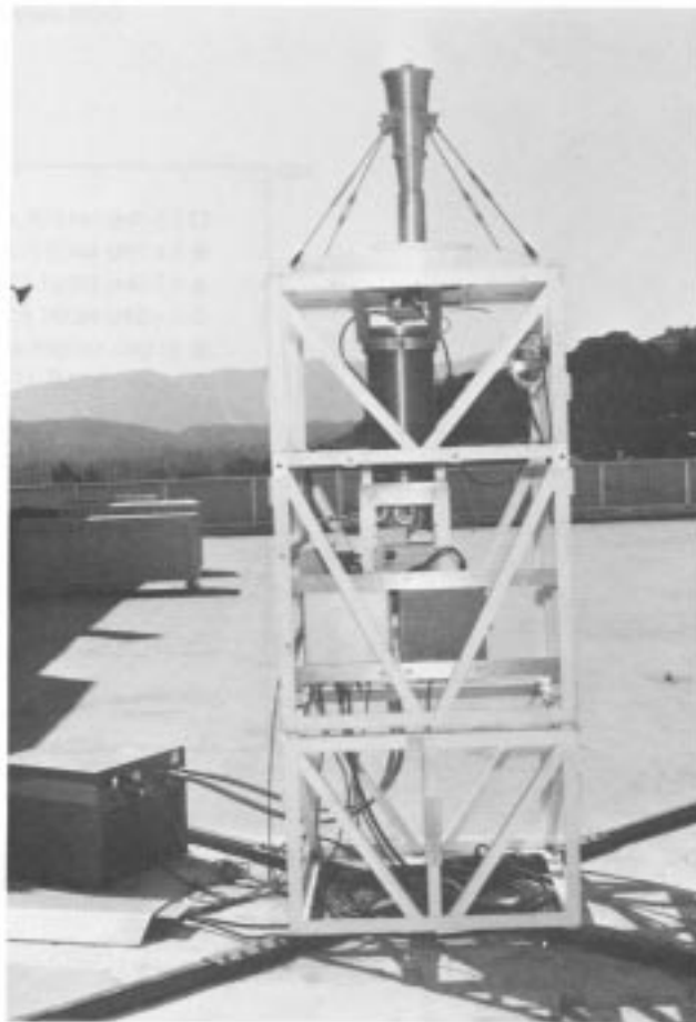
Fig. 14. A 32-GHz HEMT/CCR total power radiometer.
