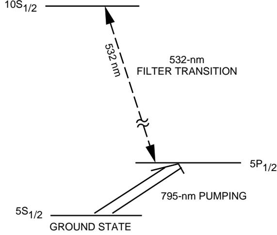
**Fig. 2. A simplified Rb 532-nm SADOFF energy-level diagram.**
