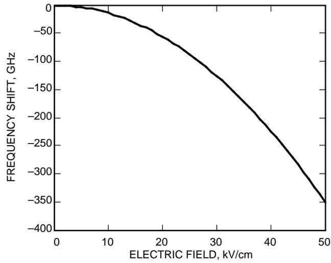
Fig. 6. Rb 532-nm SADO center frequency versus external electric field.
