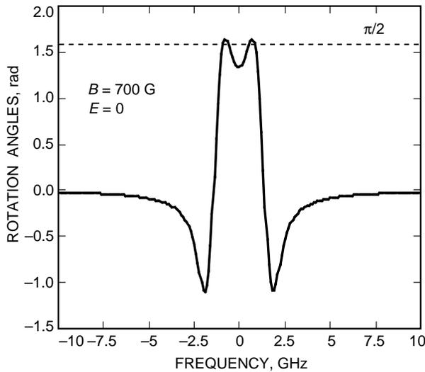
Fig. 3. Rb 532-nm SADOFF rotation angles versus frequency at  $T = 190$  deg C and  $B = 700$  G, where the horizontal axis is normalized to the frequency shift from the Rb 532-nm transition.
