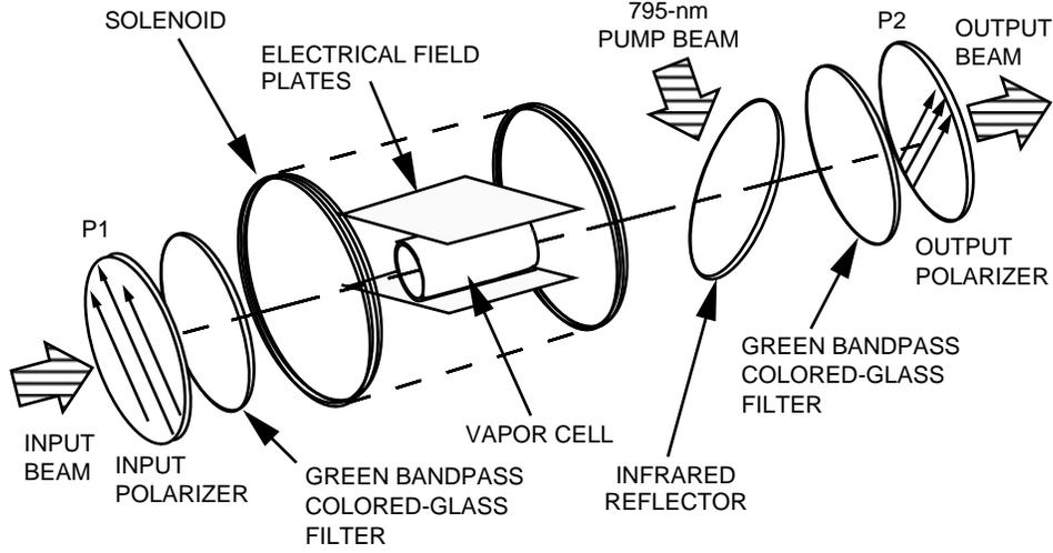
Fig. 1. The basic structure of an Rb 532-nm SADO.
