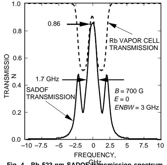
Fig. 4. Rb 523-nm SADOFF transmission spectrum at  $T = 190$  deg C,  $B = 700$  G, and  $E = 0$  kV/cm, where the horizontal axis is normalized to the frequency shift from the 532-nm transition.
