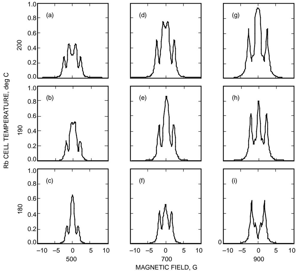
Fig. 7. Rb 532-nm SADO transmission spectrum at  $E = 0$  and at (a) 500 G, 200 deg C,  $ENBW = 3.9$  GHz; (b) 500 G, 190 deg C,  $ENBW = 3.2$  GHz; (c) 500 G, 180 deg C,  $ENBW = 2.0$  GHz; (d) 700 G, 200 deg C,  $ENBW = 4.2$  GHz; (e) 700 G, 190 deg C,  $ENBW = 3.0$  GHz; (f) 700 G, 180 deg C,  $ENBW = 3.2$  GHz; (g) 900 G, 200 deg C,  $ENBW = 4.0$  GHz; (h) 900 G, 190 deg C,  $ENBW = 3.4$  GHz; and (i) 900 G, 180 deg C,  $ENBW = 3.0$  GHz.
