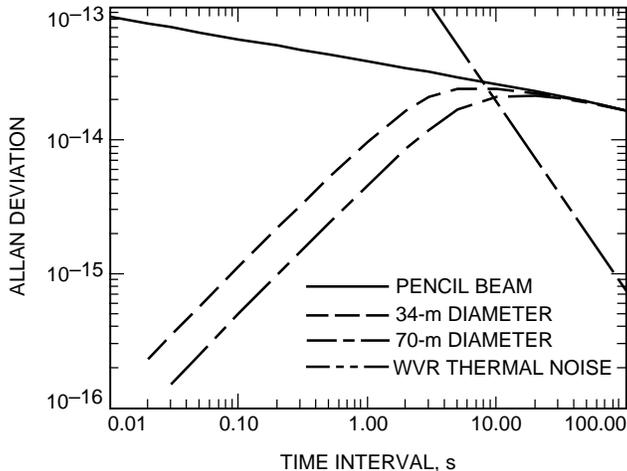
**Fig. 1.** The Allan deviation calculated for a pencil beam antenna and for antenna diameters of 34 and 70 m is shown as a function of time interval for typical Goldstone conditions and the zenith direction. The Allan deviation at other elevation angles will be somewhat larger, increasing by a factor of 1.8 at a 10-deg elevation angle. The thermal noise from a WVR with the characteristics expected for the Cassini radio science calibration system is included.
