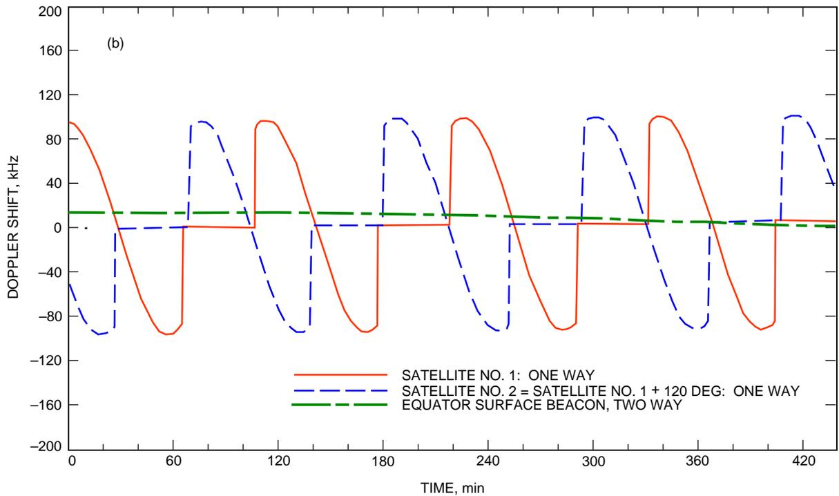
**Fig. B-1. As viewed from Earth for two 300-km altitude Mars orbiters and a lander beacon at the Mars equator, with an 8450-MHz transmission frequency: (a) the Doppler profile and (b) an enlargement of the profile.**
