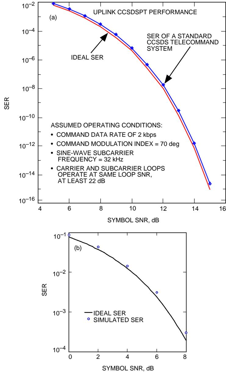
**Fig. 6. Performance of system option no. 1: (a) the SER for a standard CCSDS telecommand system and (b) the simulated SER for a typical SFDMA telemetry system.**
