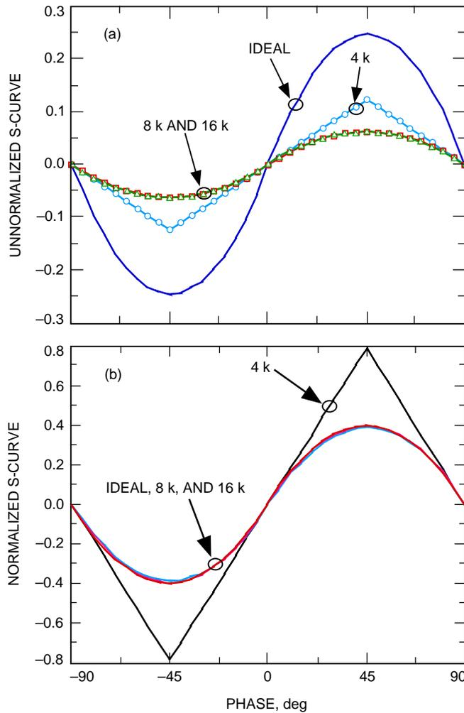
**Fig. 15. S-curves for tracking 4-, 8-, and 16-kHz sub-carriers: (a) unnormalized and (b) normalized.**
