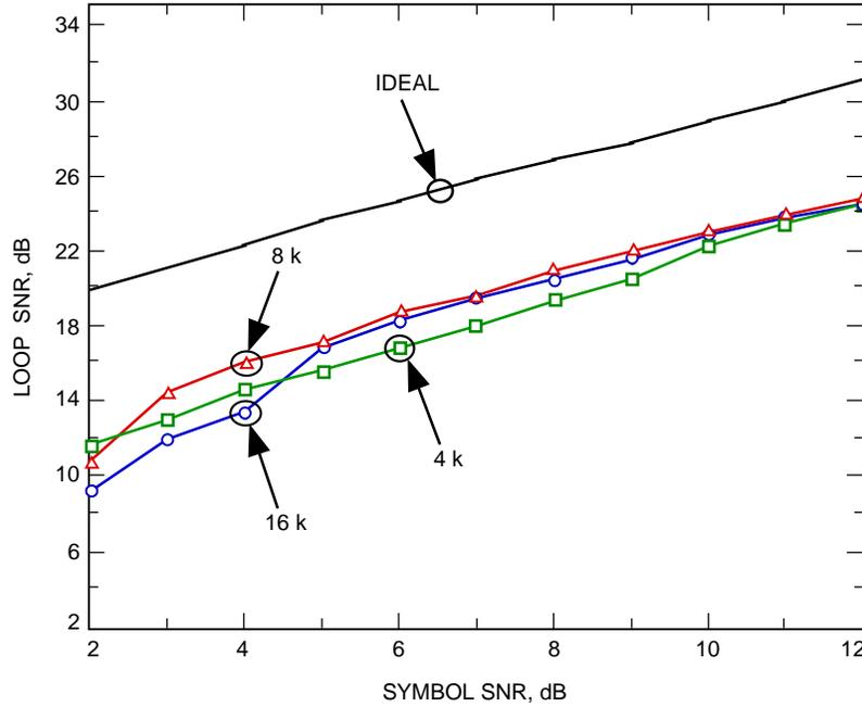
Fig. 16. Unnormalized S-curves for tracking 4-, 8-, and 16-kHz subcarriers.
