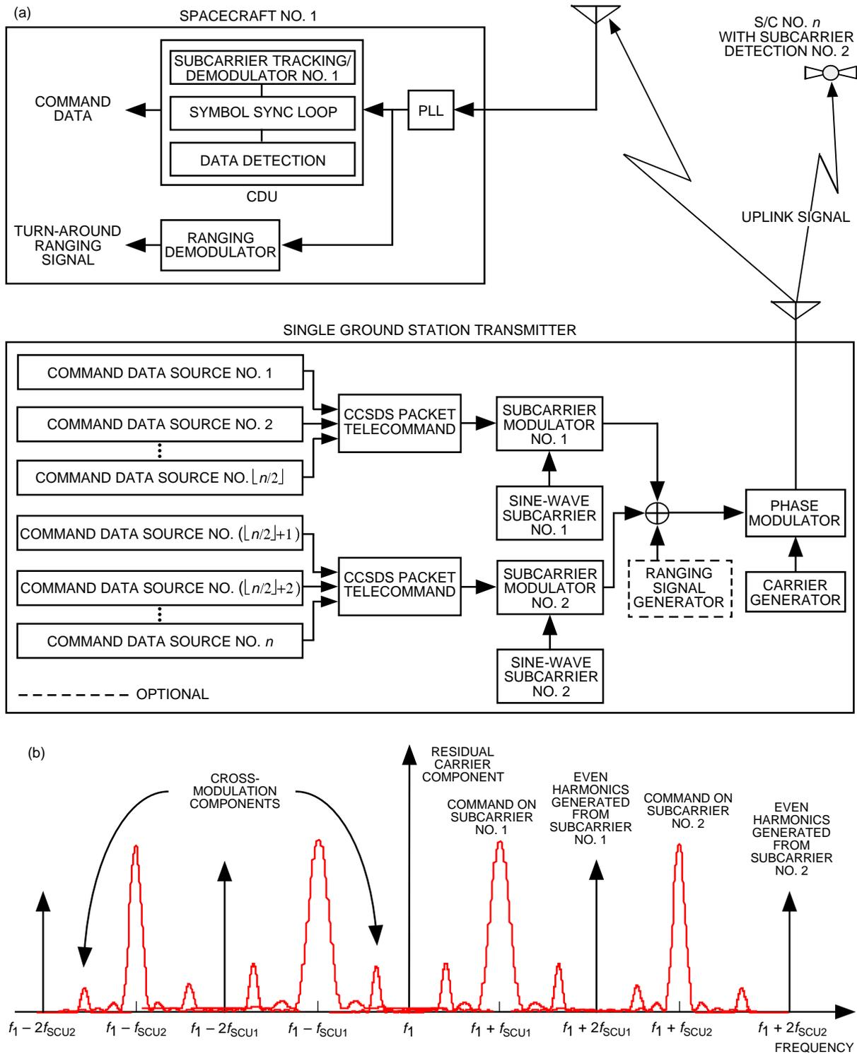
Fig. 7. System option no. 2: (a) a simplified block diagram for the SFDM uplink system and (b) the spectrum of the uplink signal without ranging signal.
