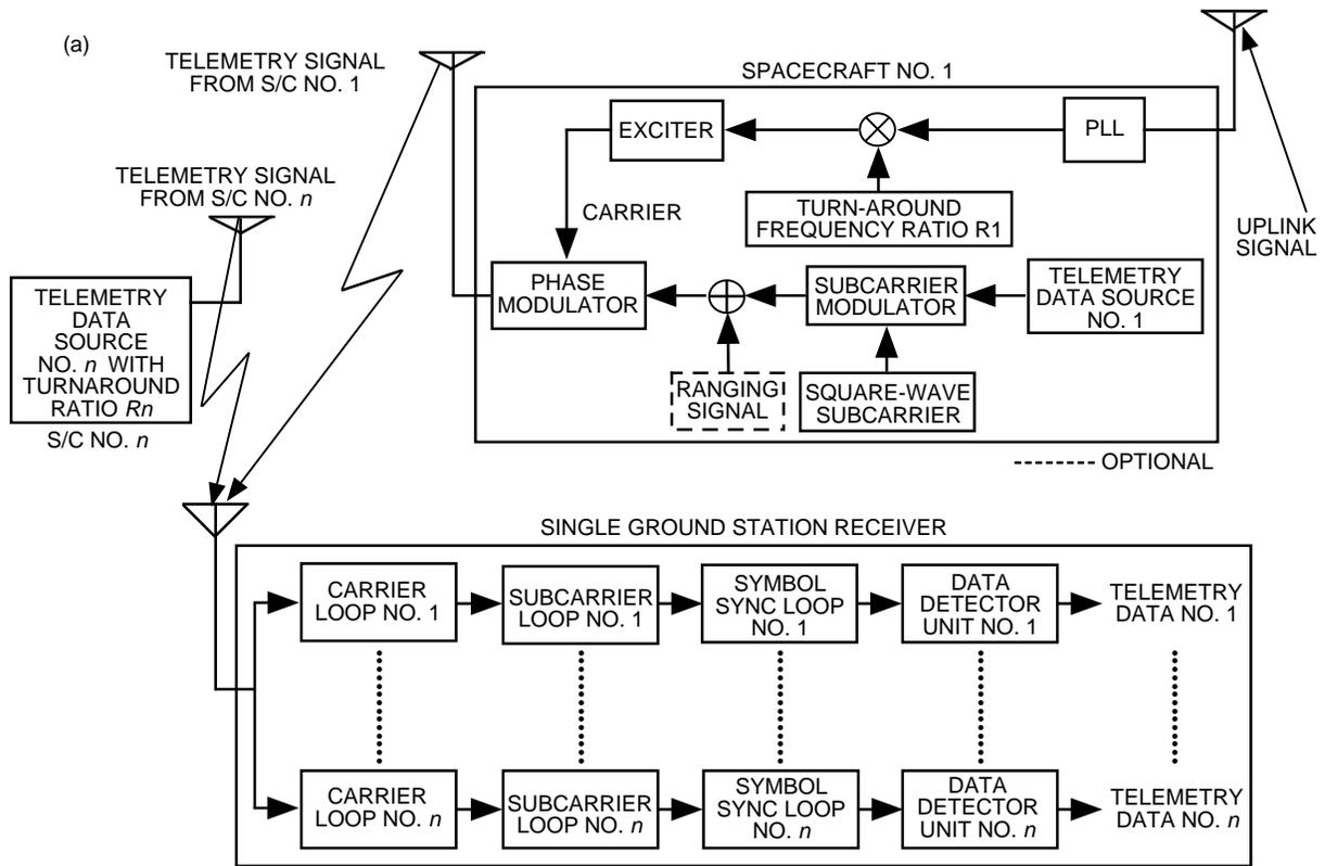
Fig. 8. System option no. 3: (a) a simplified block diagram of the CFDMA downlink system architecture with adjustable turn-around frequency ratio and (b) the spectrum of the downlink signal without ranging signal.
