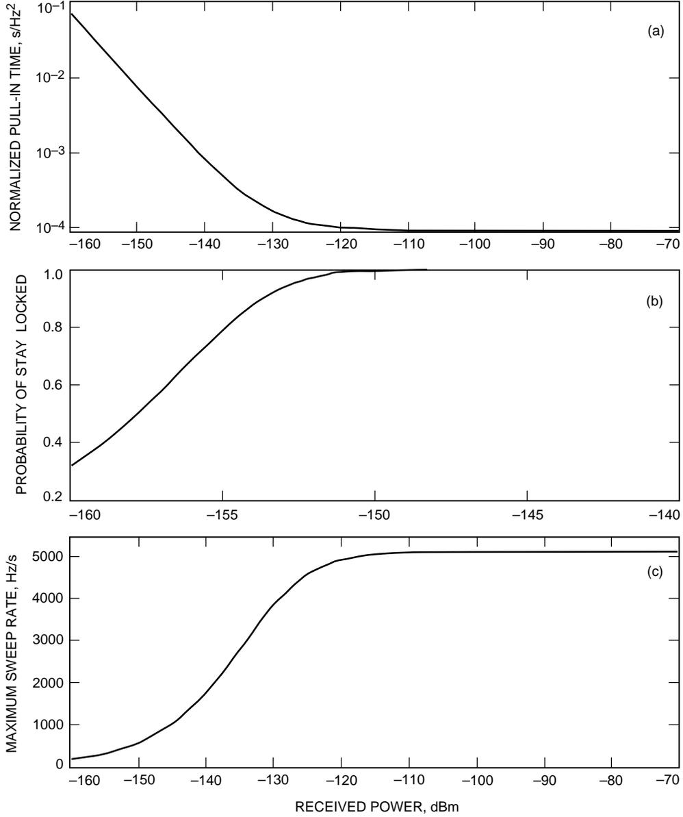
**Fig. 5. Uplink carrier acquisition performance: (a) normalized pull-in time, (b) probability of staying in lock, and (c) maximum sweep rate.**
