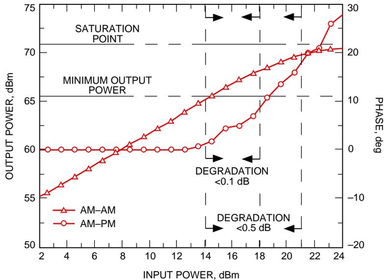
Fig. 17. Typical power amplifier characteristics for the DSN (Varian VA - 846 klystron).
