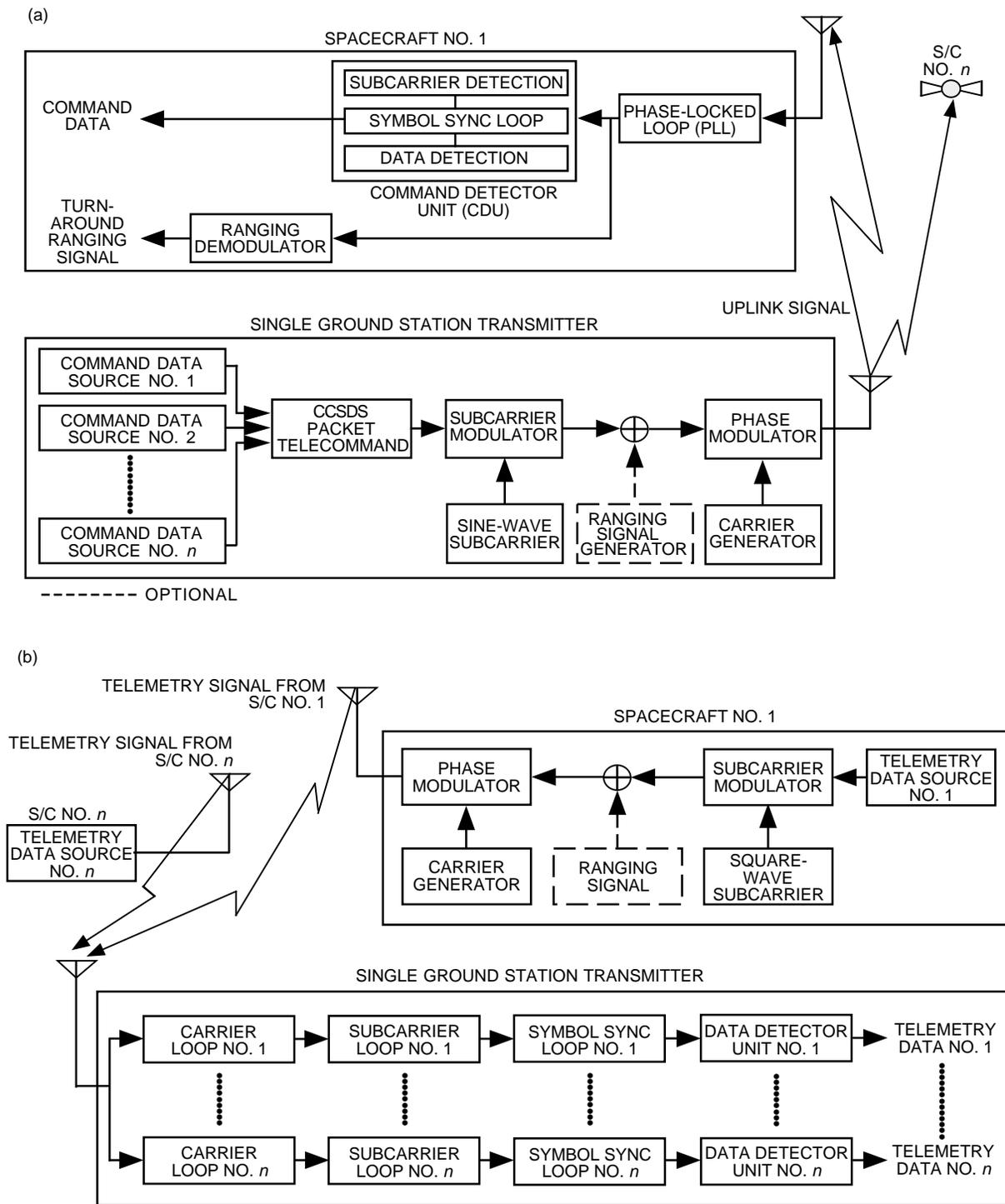
Fig. 2. System option no. 1: (a) a simplified block diagram of the CCSDSPT uplink, (b) a simplified block diagram of the SFDM downlink, (c) the spectrum of the uplink signal without the ranging signal, and (d) the spectrum of the downlink signal without the ranging signal.
