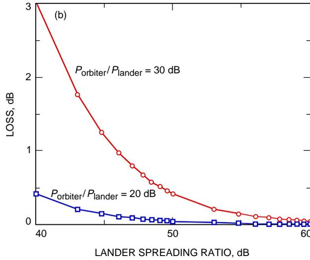
**Fig. 11. Performance of system option no. 4: (a) loss versus the spreading ratio for spacecraft at a data rate of 20 kbps and (b) the lander spreading ratio versus loss in a three-user scenario (two orbiters and one lander).**
