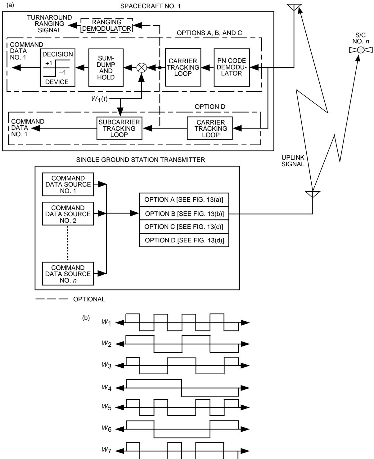
Fig. 12. System option no. 5: (a) a simplified block diagram for the CDM uplink system and (b) regular length-8 Walsh functions ( $W_0 = 1$  is not included here).
