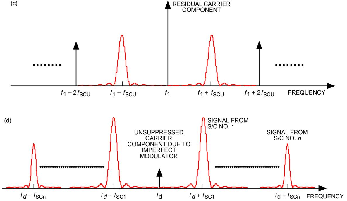
**Fig. 2 (cont'd). System option no. 1: (a) a simplified block diagram of the CCSDSPT uplink, (b) a simplified block diagram of the SFDM downlink, (c) the spectrum of the uplink signal without the ranging signal, and (d) the spectrum of the downlink signal without the ranging signal.**
