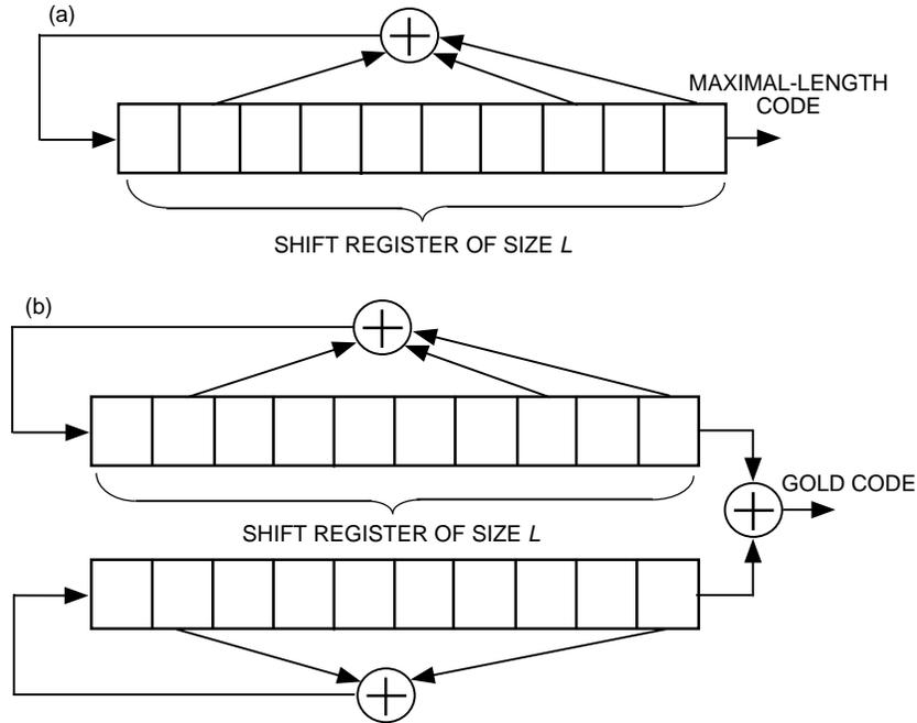
**Fig. D-1. CDMA code generators producing (a) M-sequences and (b) Gold sequences.**
