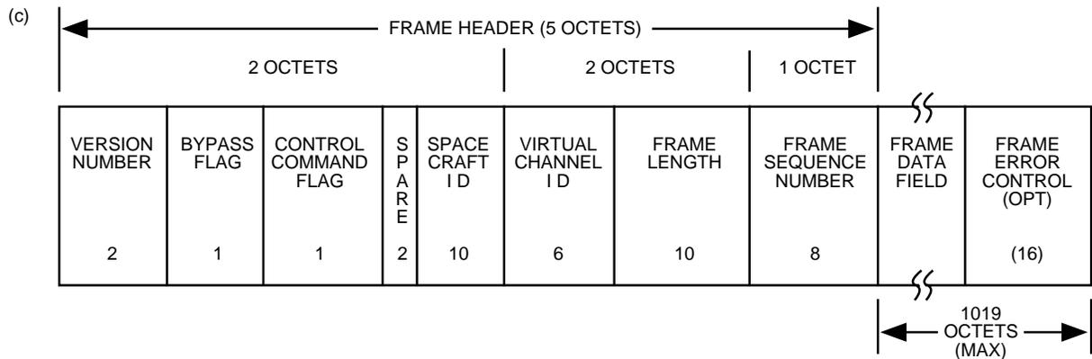
Fig. 3. Telecommand (a) data structure, (b) code block format, and (c) transfer frame format (1 octet is an 8-bit data string).
