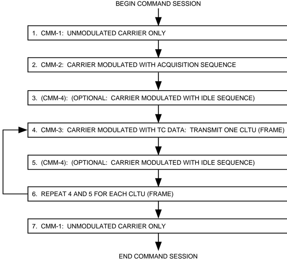
Fig. 4. The recommended carrier modulation mode (CMM) sequence on the physical layer.
