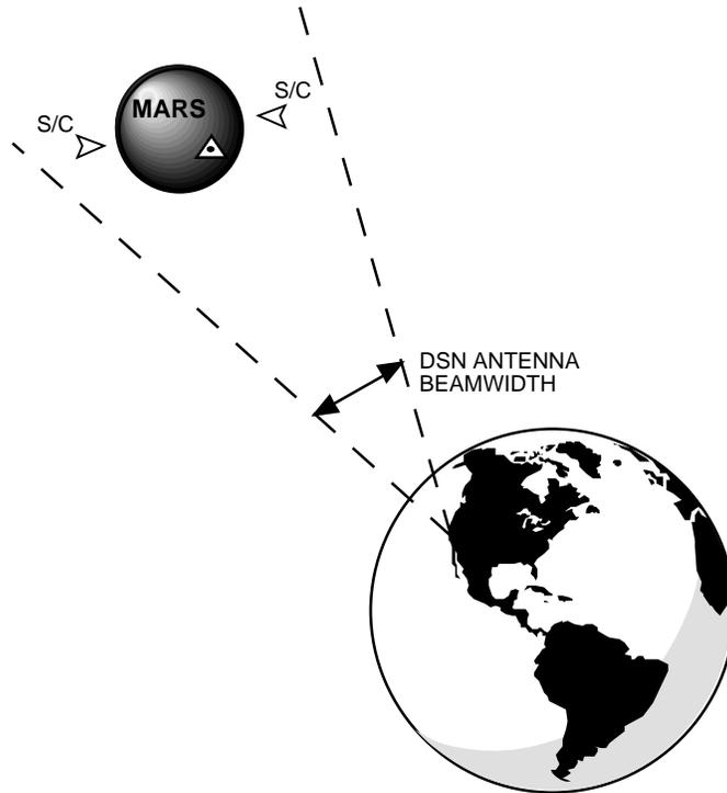
**Fig. 1. A typical scenario for multiple S/C support with a single DSN ground antenna.**
