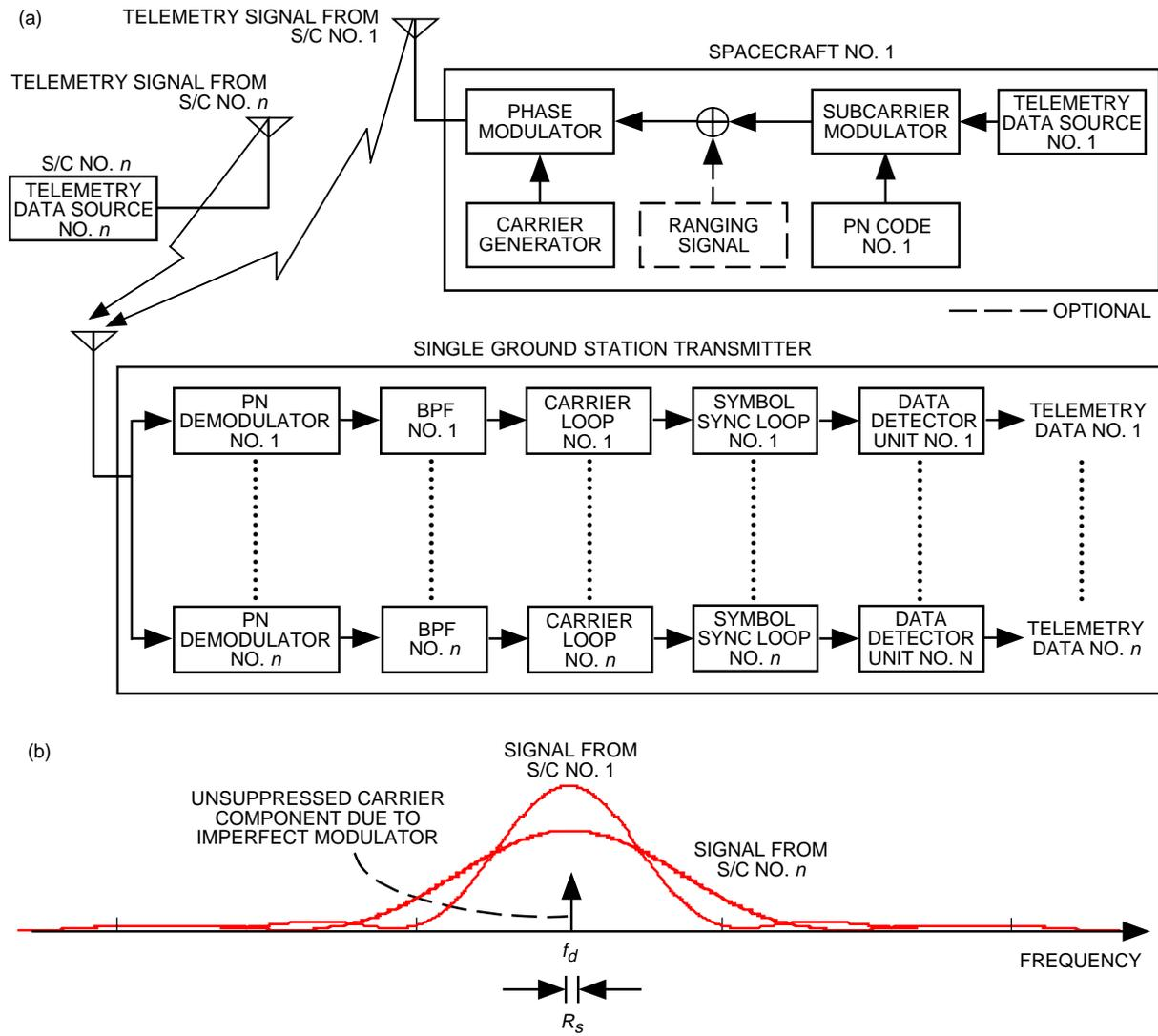
**Fig. 10. System option no. 4: (a) a simplified block diagram of the CDMA downlink system architecture and (b) the spectrum of the downlink signal without ranging signal (where  $R_s$  is the telemetry symbol rate).**
