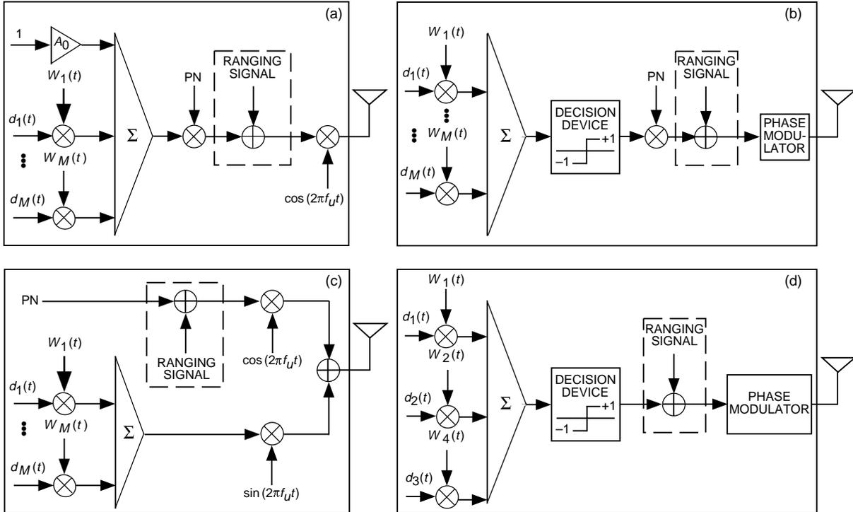
Fig. 13. The options for CDM using Walsh–Hadamard code: (a) option A, (b) option B, (c) option C, and (d) option D (an example of a three-user case).
