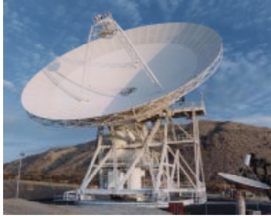
Fig. 3. DSS 13, the DSN's 34-m research and development antenna.
