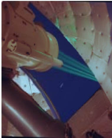
Fig. 6. The multibeam laser uplink from the Table Mountain 0.6-m telescope to the ETS-VI spacecraft during the Ground-to-Orbit Lasercom Demonstration (GOLD).
