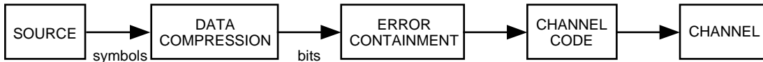
Fig. 1. Block diagram for a communications system using data compression with error containment.
