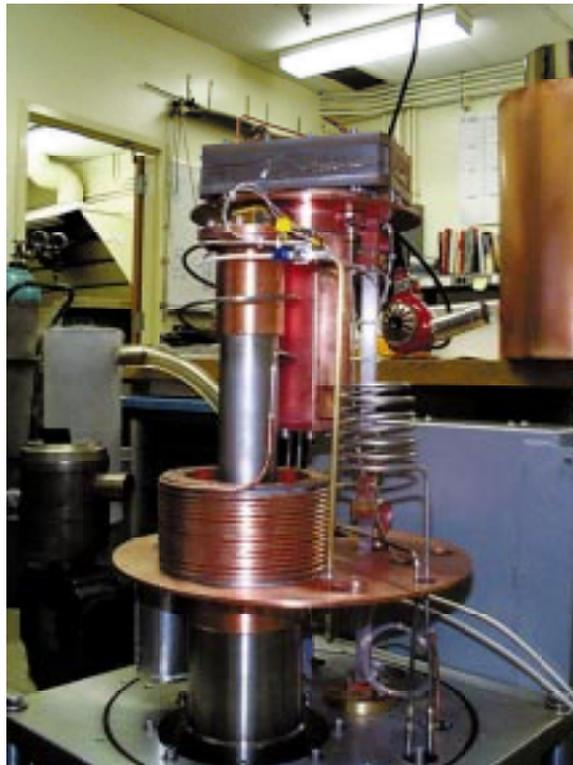
Fig. 1. The maser installed on the GM cryocooler.
