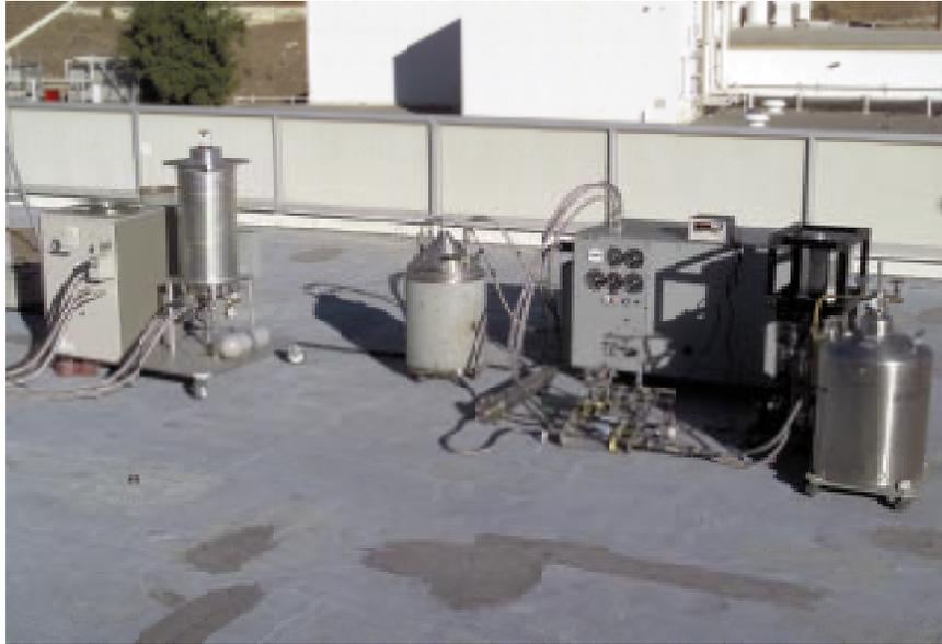
**Fig. 3. The GM-cooled maser system (left) and the current DSN JT-cooled maser system (right).**
