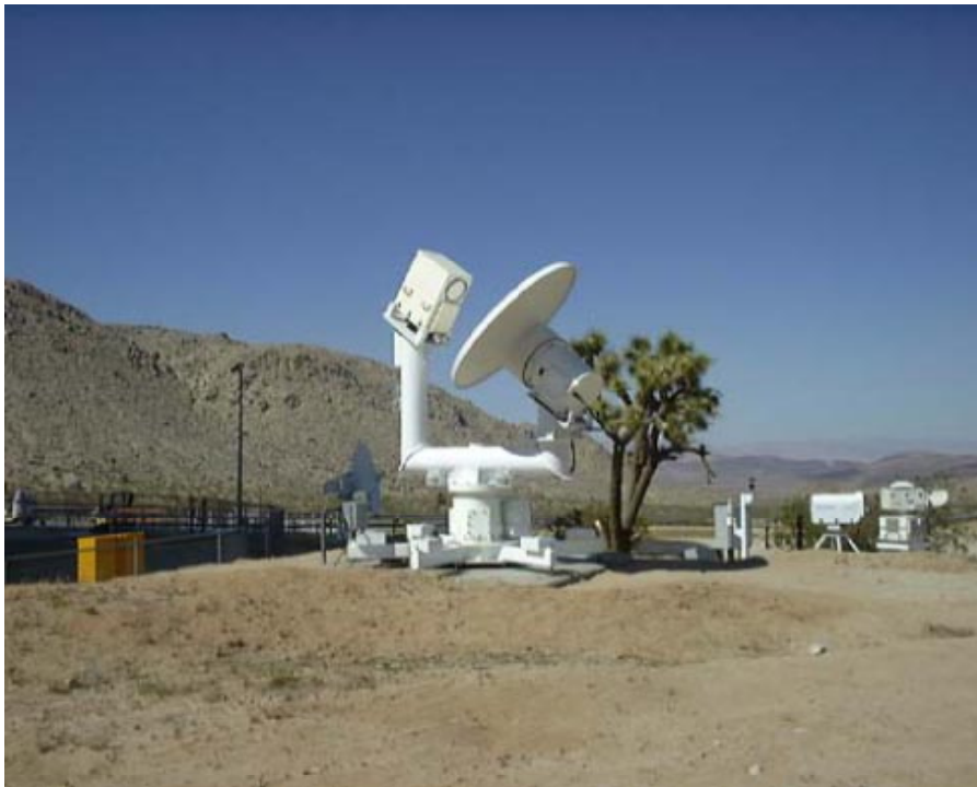
Fig. 1. The media calibration subsystem at DSS 13 in Goldstone, CA. The new advanced WVR is seen in the center, and the MTP is shown in the background to the right.
