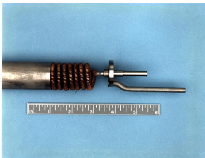
Fig. 8. JT heat exchanger detail.
