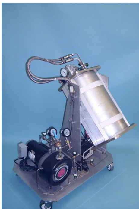
Fig. 7. A view of the cooler tipped on the gimbal.
