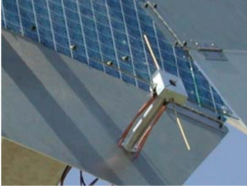
Fig. 5. The cross-dipole antenna on the MER solar array.
