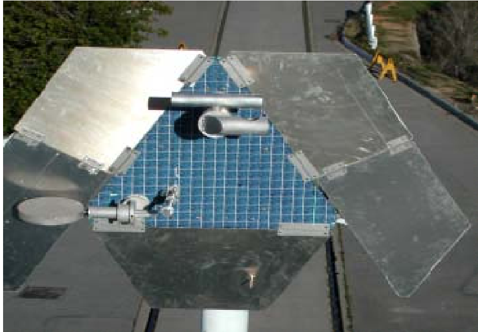
Fig. 1. The monopole antenna on the new MER mock-up.
