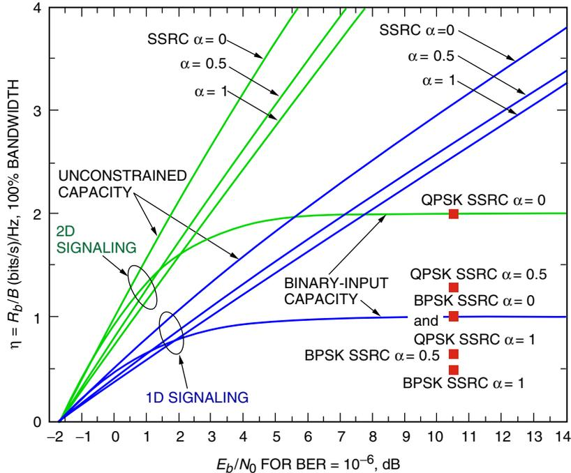
Fig. 4. Effect of filtering on unconstrained and binary-input capacity.
