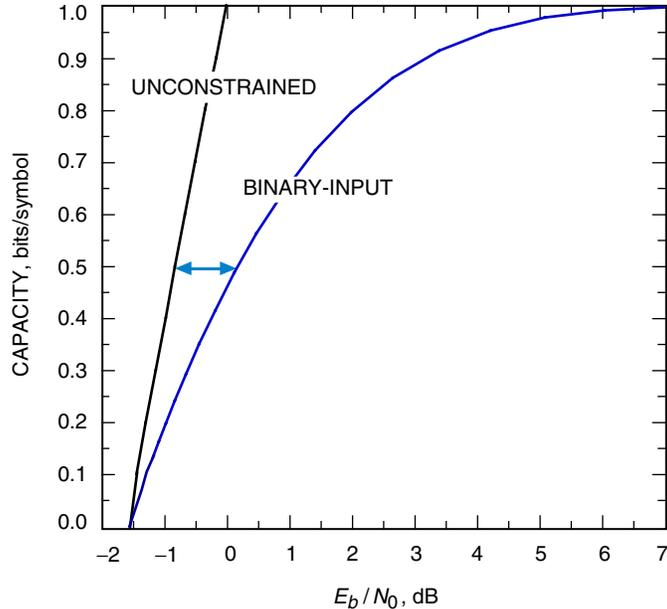
**Fig. 1. Capacity of the additive white Gaussian noise channel with unconstrained and binary-input signaling.**
