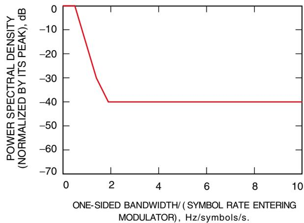
**Fig. 9. Mask of modified SFCG Recommendation 21-4, provisional.**
