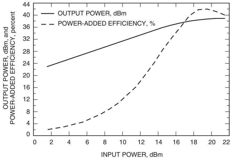
Fig. 10. SSPA input-to-output power and power-added efficiency characteristics.
