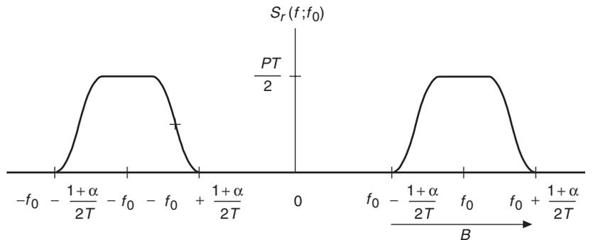
Fig. 7. Raised cosine spectrum.
