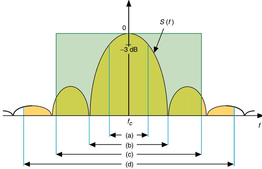
**Fig. 2. Some of the possible measures for spectral efficiency: (a) half-power bandwidth, (b) null-to-null bandwidth, (c) equivalent noise bandwidth, and (d) fractional power containment bandwidth.**
