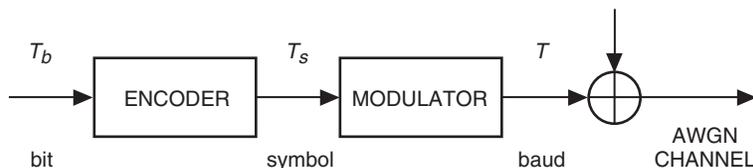
Fig. 3. Model for coded modulation systems.
