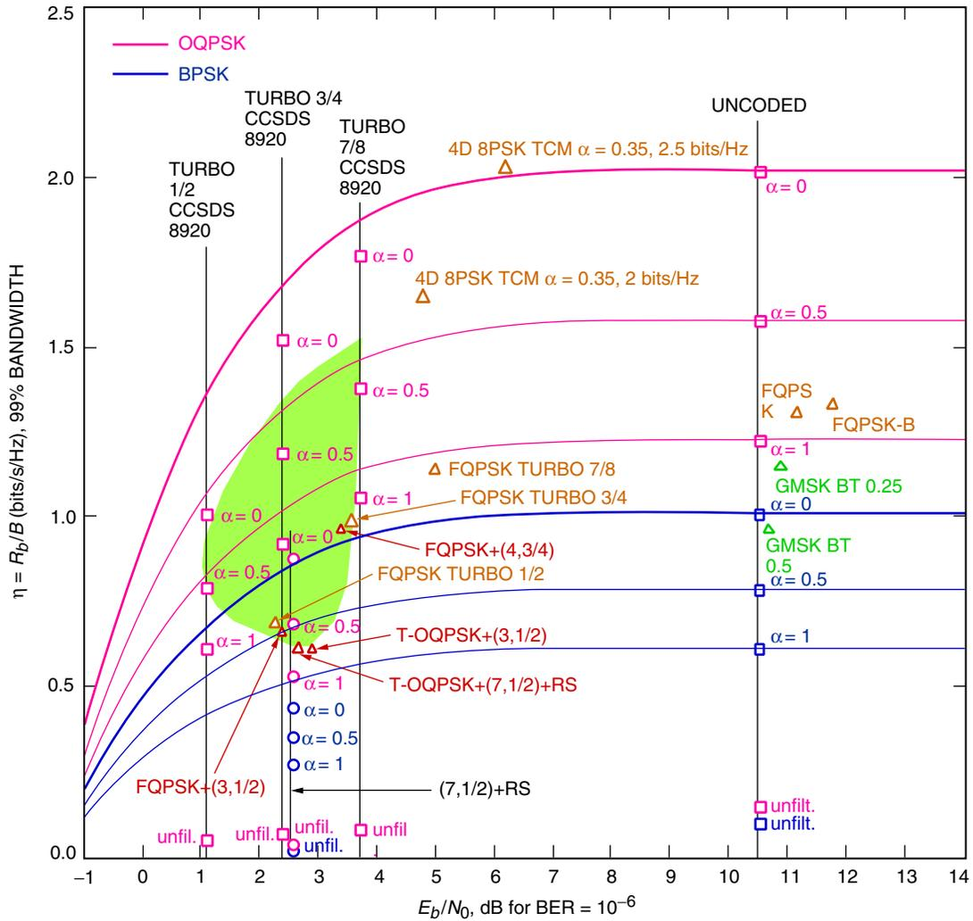
**Fig. 8. Comparison of several coded modulation schemes showing the region of interest for Mars missions.**
