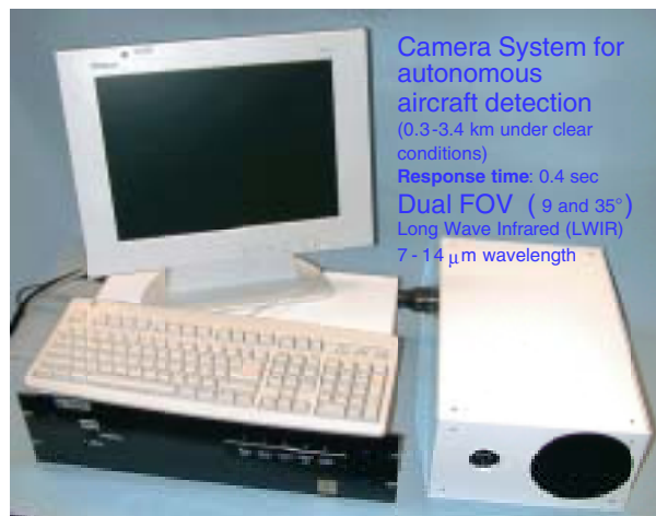
Fig. 4. Image Labs International Tier-1 aircraft avoidance system consists of two LWIR cameras (a wide field of 35 deg \times 46 deg and a narrow field of 12 deg \times 9 deg).
