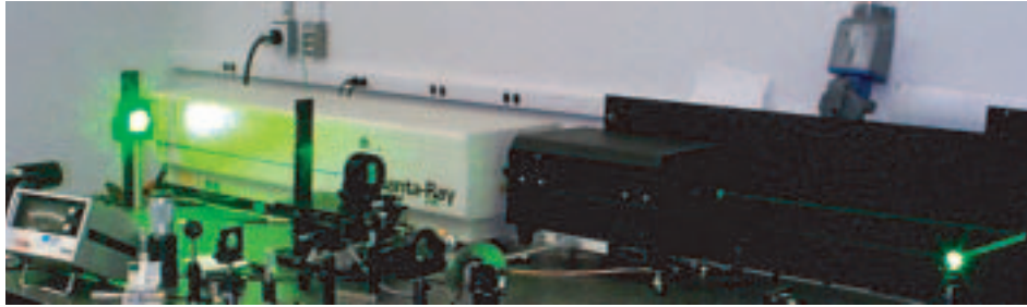
Fig. 3. Picture of a Q-switched Nd:YAG laser beam taken by an operator using OD-6 safety goggles. The laser operates at a variety of pulse-repetition rates between 1 Hz and 51 Hz.
