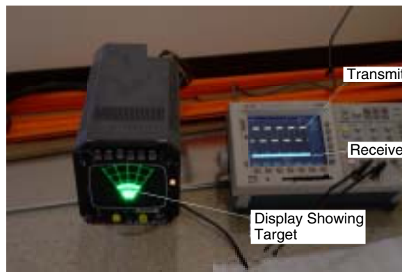
Fig. 7. Transmit and receive signals from the display unit.
