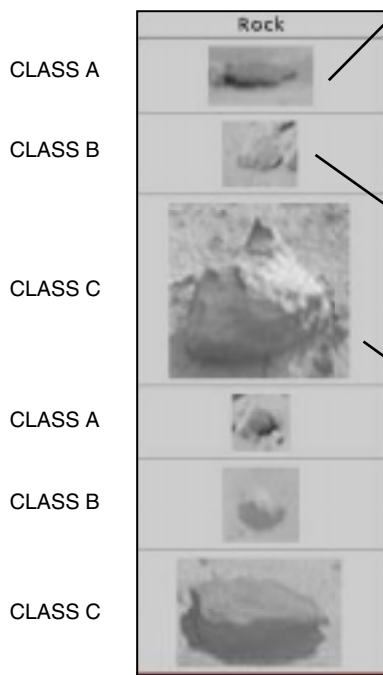
Fig. 5. Prioritized ranking of rocks for three clusters of rocks. Using the representative target prioritization technique ensures that images containing the most representative rock of each class have the highest priority for downlink.
