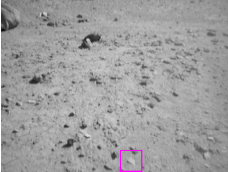
Fig. 4. Detection of a significant novel rock. One of the most novel rocks detected in the test data set is the rock indicated in this image. The marked rock is a piece of petrified wood that is extremely interesting to scientists. Unfortunately, during the course of the FIDO field test, the petrified wood was not identified by the remotely located geologists.
