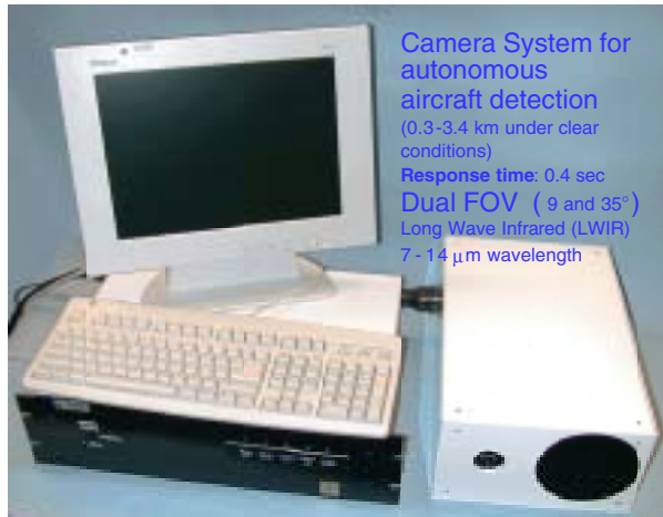
Fig. 7. Image Labs International LWIR detection system for Tier 1 aircraft avoidance.
