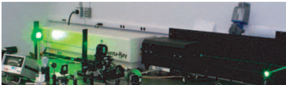
Fig. 3. Picture of a Q-switched Nd:YAG laser beam. The laser operates at a variety of pulse-repetition rates between 1 and 50 Hz.
