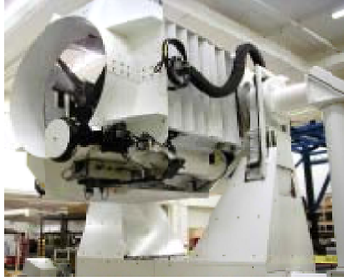
Fig. 2. The OCTL telescope undergoing testing at the vendor's facility. The louvered baffles, the 20-cm acquisition telescope, and the M4 and M5 coudé path tube are shown.
