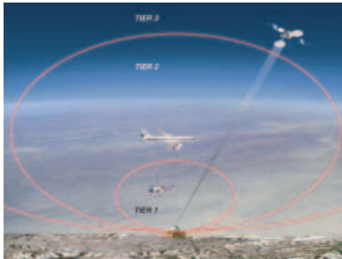
Fig. 6. Three JPL-defined safety tiers for ground-to-space laser beam propagation.
