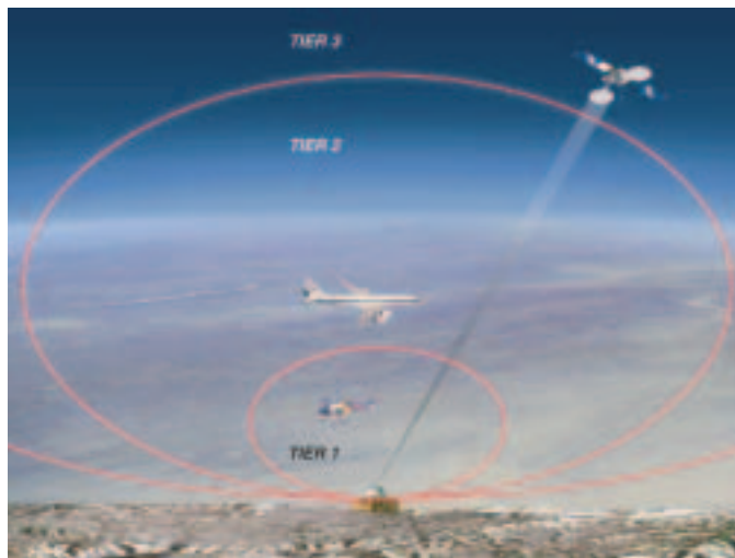
Fig. 1. The three JPL-defined safety tiers for ground-to-space laser beam propagation from the OCTL. Reprinted from [2].
