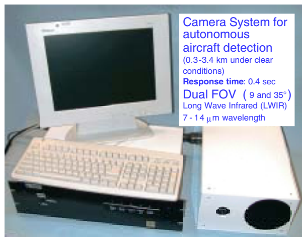
Fig. 2. Image Labs International LWIR detection system for Tier-1 aircraft avoidance. Reprinted from [2].
