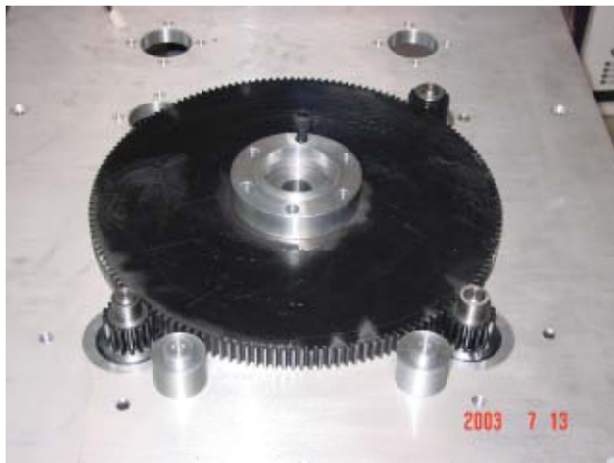
Fig. 2. Test-bed bull gear with two pinions.
