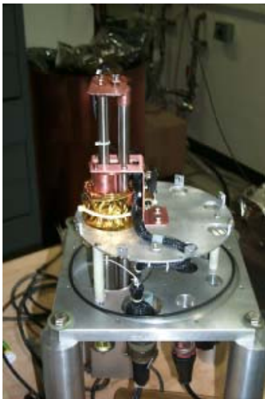
Fig. 3. GB-15 cryocooler installed.
