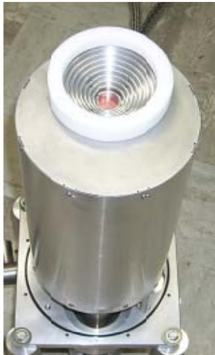
Fig. 6. Aluminum radiation shield installed.
