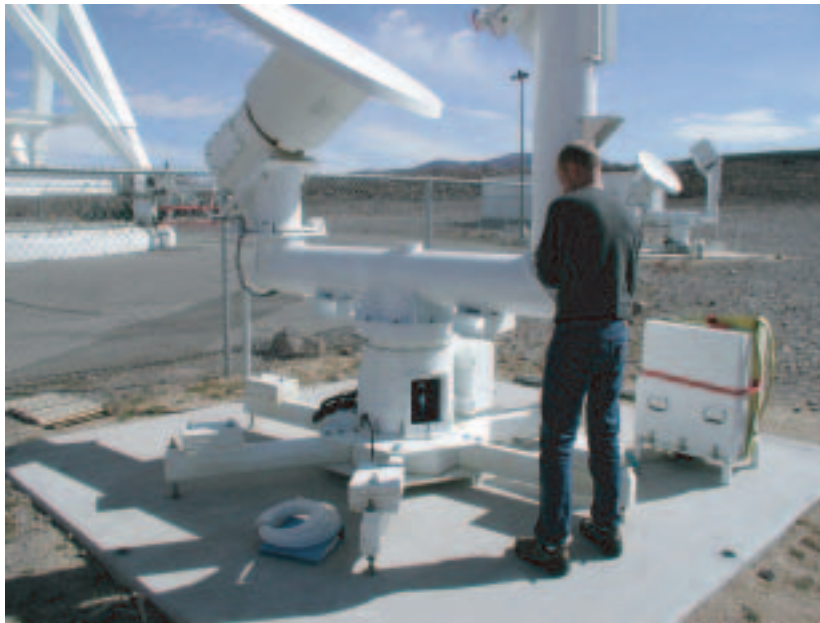
Fig. 1. One of the two Advanced Water Vapor Radiometers at DSS 25.
