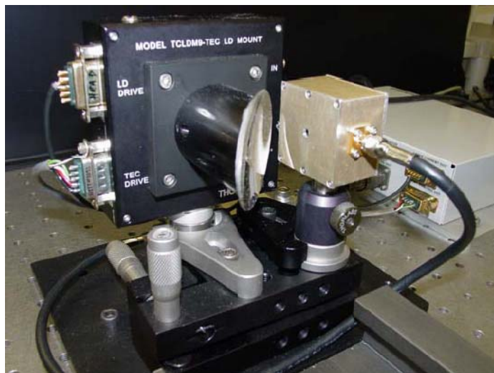
Fig. 2. Laser transmitters and receiver.
