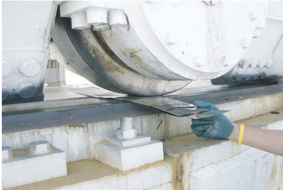
Fig. 14. The azimuth wheel crosses a 1-mm shim.
