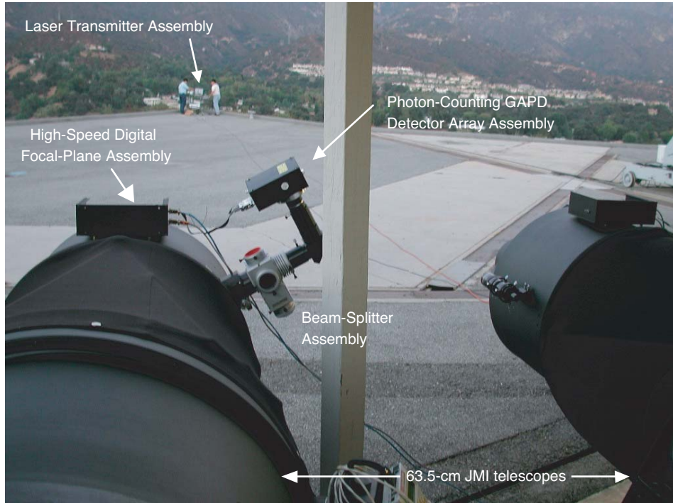
Fig. 8. Experimental setup on the JPL Mesa test range, for reception of PPM signals.
