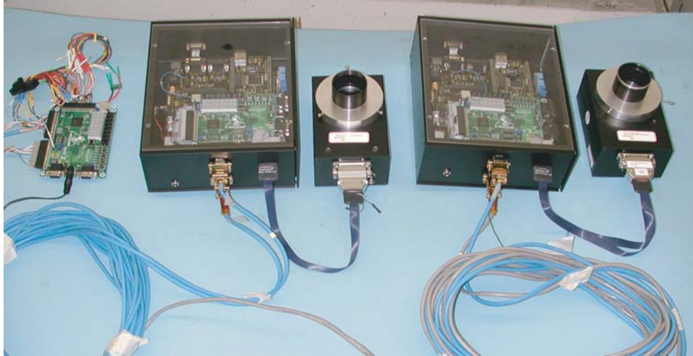
Fig. 6. Complete OACEA, before installation on 63.5-cm telescopes, including a peak detector modules, focal-plane electronics, high-speed 4-bit LVDS cable assemblies, and adaptive delay compensation and combining board.
