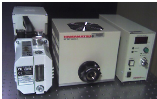
Figure 3. Near-infrared photomultiplier tube with vacuum pump and voltage- and temperature-control electronics.
