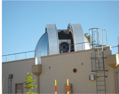
Figure 1. Optical Communications Telescope Laboratory with the 1-m elevation/azimuth telescope shown through open dome.
