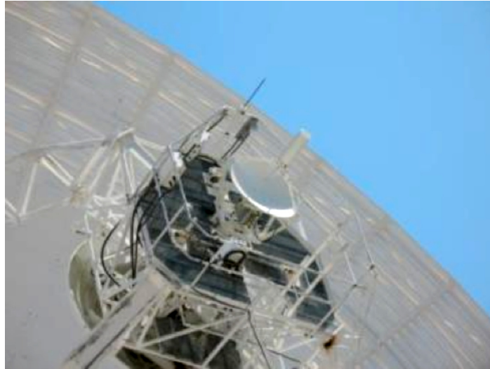
Figure 15. Acquisition aid mounting on 34-m BWG antenna subreflector.
