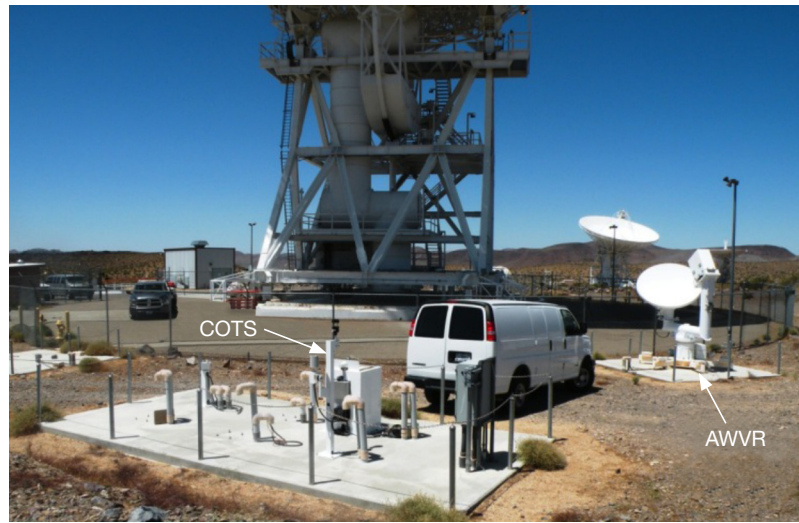
Figure 6. COTS and AWVR instruments installed at DSS-25.
