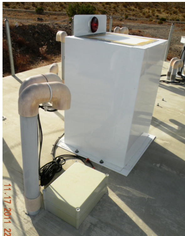
Figure 4. Radiometer in enclosure installed at DSS-25.
