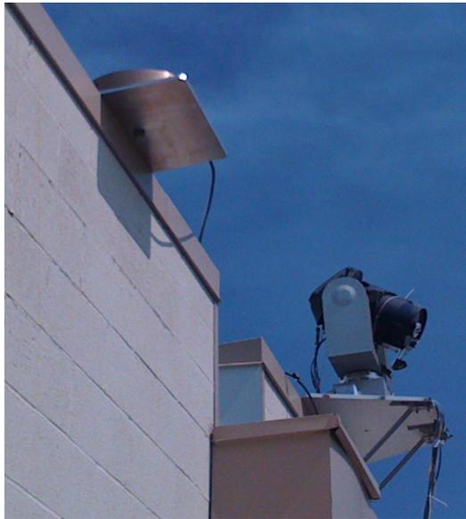
Figure 3. GPS choke-ring antenna installed next to ALURE at the Table Mountain facility.
