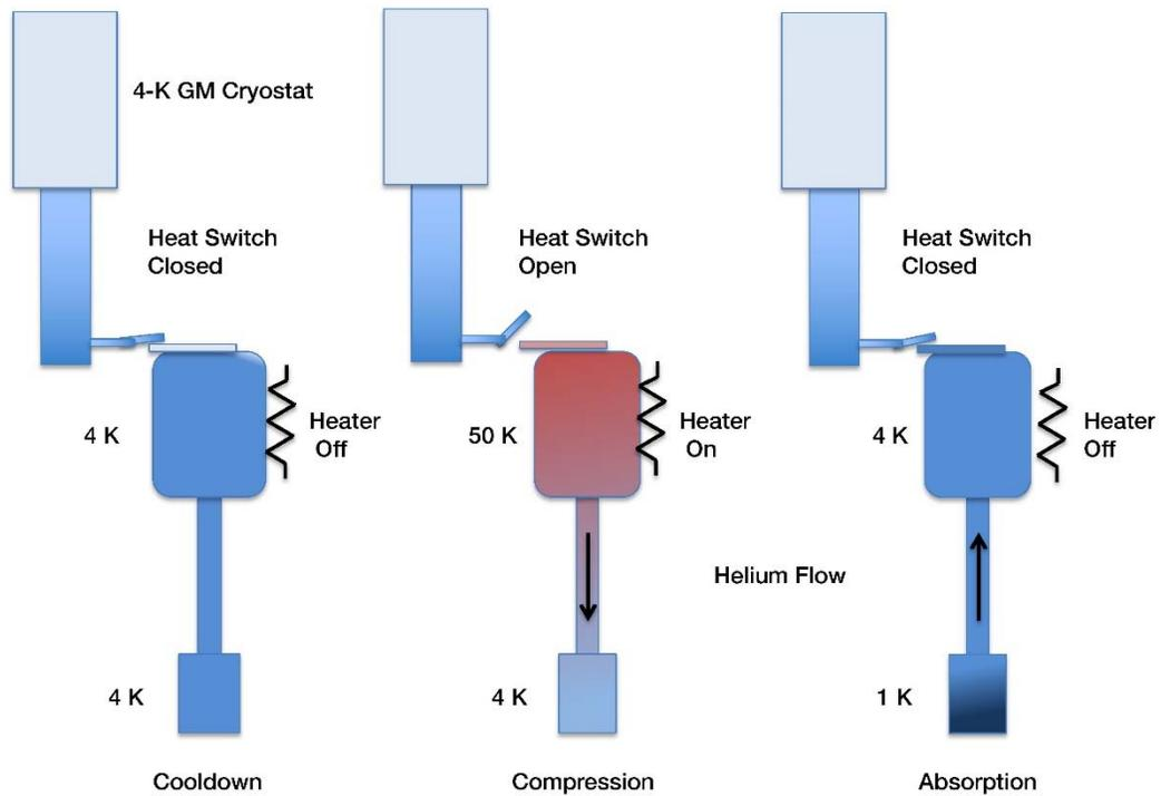
Figure 1. Cartoon showing 1-K cryostat operating cycle working with 4-K GM cryostat.
