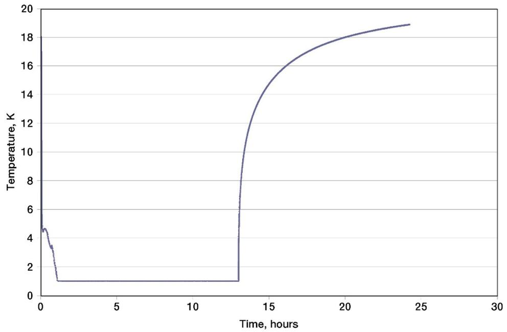
**Figure 3. Operating temperature with cryostat operating at 20 deg elevation.**
