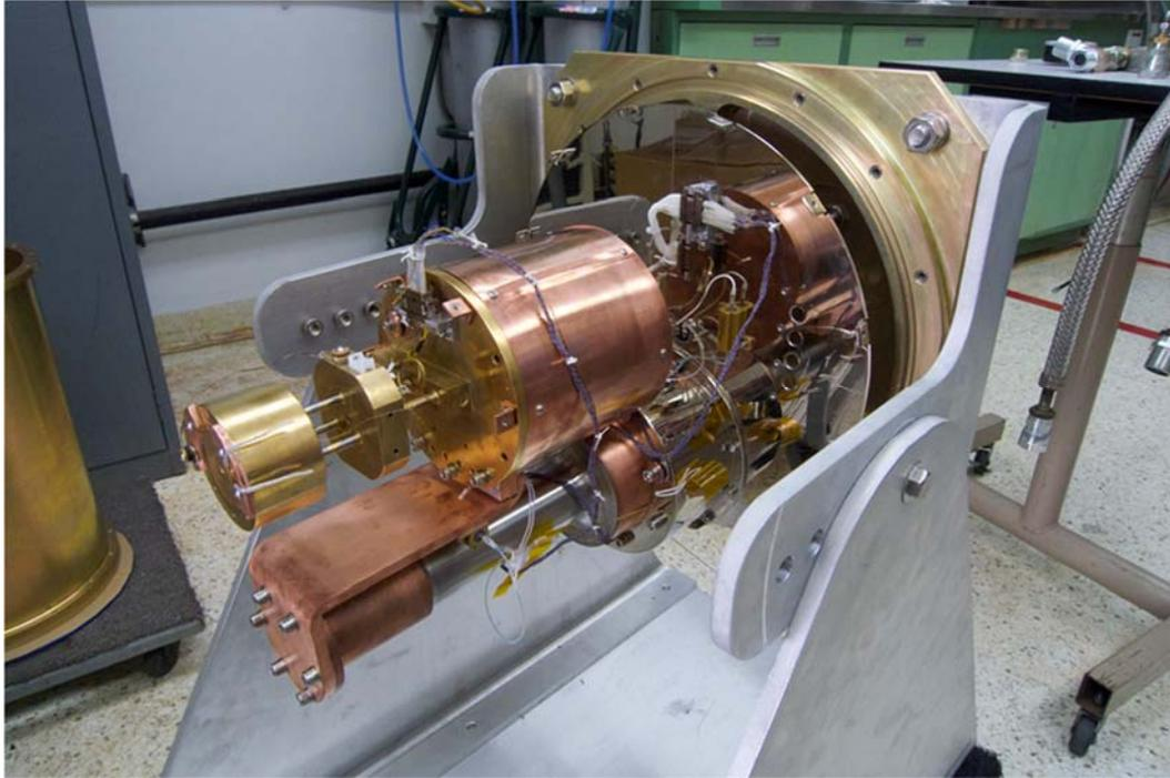
Figure 2. Cryostat with vacuum housing and shield removed.
