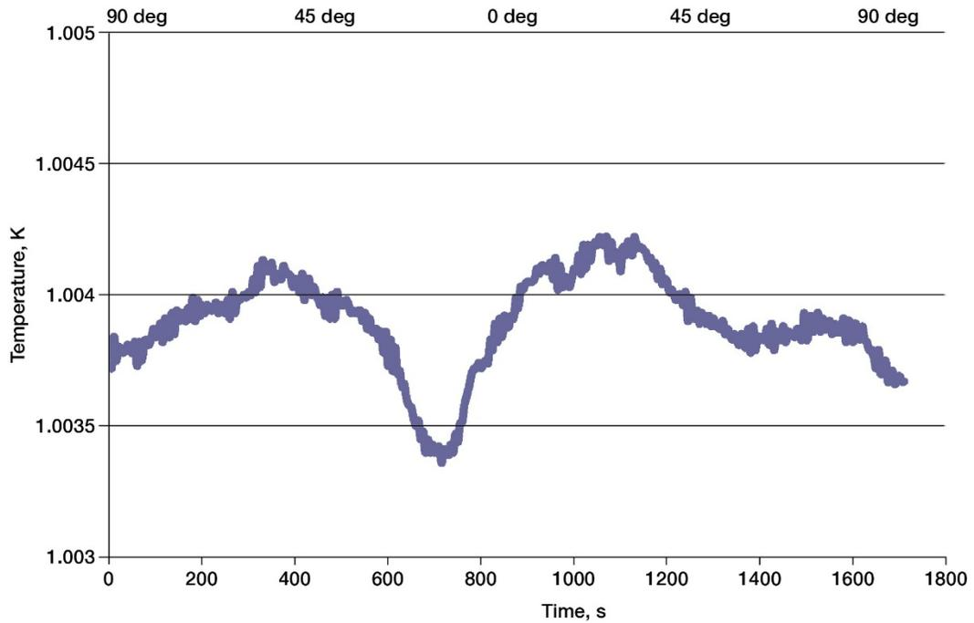
Figure 5. Temperature variation during 90–0–90 deg tilt test.
