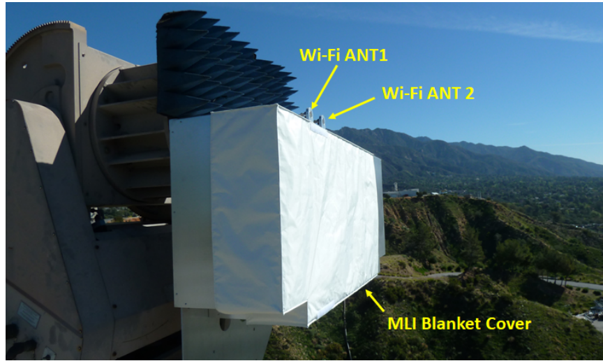
Figure 35. Wi-Fi antenna gain test with ECOSTRESS payload mockup and MLI blanket
