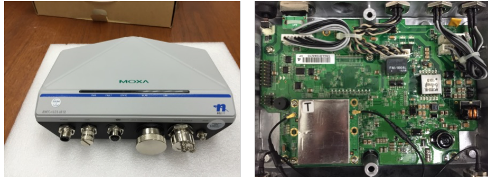
Figure 24. Left: Moxa AWK-4131 COTS Enclosure. Right: AWK-4131 Wi-Fi board after disassembly.
