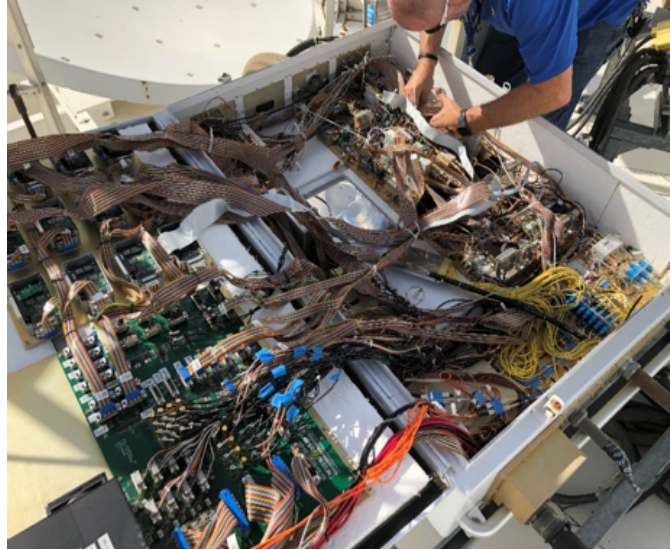
Figure 6. DSS-28 receiving equipment upgraded at GDSCC in order to receive 7150 MHz echoes from the Tycho region on the Moon.
