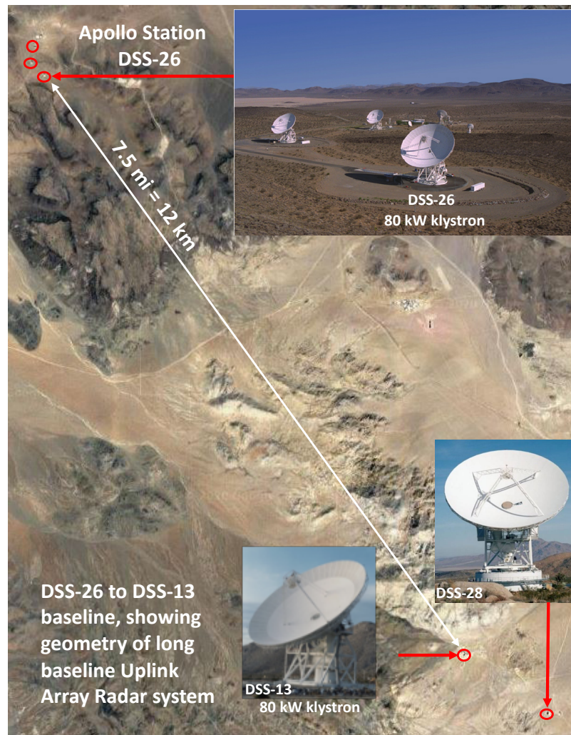
Figure 4. Geometry of Apollo Station, DSS-13, and DSS-28 at the Goldstone Deep Space Communications Complex.
