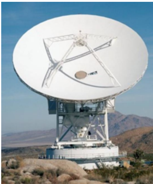
Figure 3. The 34 m GAVRT antenna at DSS-28 that received the radar echoes from the Moon in bistatic configuration.
