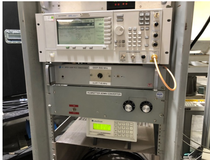
Figure 5. X-band (7150 MHz) to 320 MHz IF downconverter assembly in the DSS-13 antenna's pedestal room.
