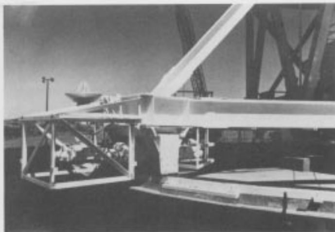
Fig. 7. Azimuth wheel and drive motors, DSS 15
