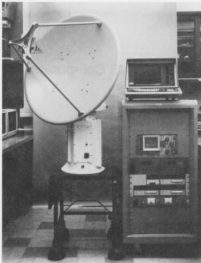
Fig. 7. SETI RFI spectral surveillance system
