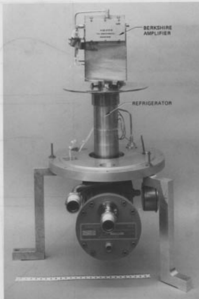
Fig. 2. Berkshire amplifier mounted on the 15-K station of the FET/CCR assembly (vacuum jacket and radiation heat shields removed)
