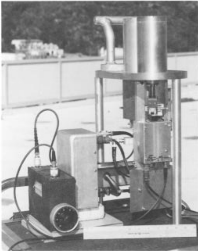
Fig. 2. Dicke radiometer front end.
